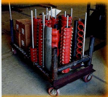
Prefabbed pipe sections are loaded and sent to jobsites on carts, eliminating banding and unbanding tasks.
